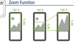
Using the included remote control, the upper image can be enlarged in 10 steps. This means that the individual image section is optimally adapted to the application during setup.
