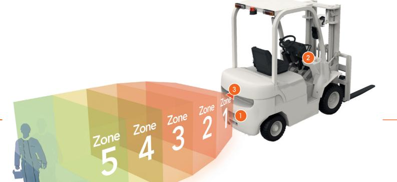
Depending on the requirements, individual settings in detection depth and width are possible Contact us
